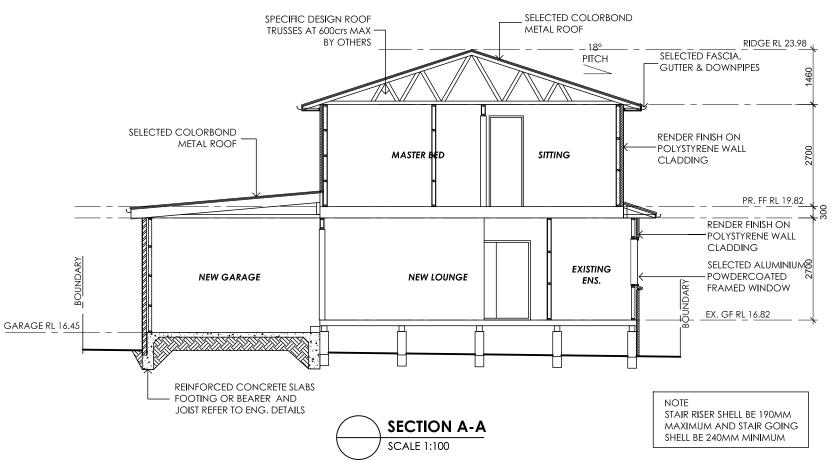
TIMBER FRAMING TO AS 1684 "RESIDENTIAL TIMBER FRAMED CONSTRUCTION CODE"
